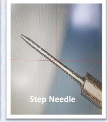
EJECTOR Needles functions as a media to push or eject the die off the adhesive (mylar) tape during the die attach process. We recommend our polished and critically machined pins made from specially recommended materials – especially to **eliminate issues** like 'die marks' (cracks) and 'die floating'...
