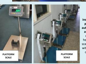
Platform Scale is an industrial weighing instrument consisting of a platform coupled to an automatic system of levers and adjustable weights, used to weigh large or heavy objects. A platform scale is a weighing machine with a platform to hold the object or objects being weighed.
